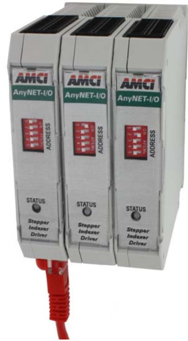
Figure R1.1 AnyNET-I/O Module Stack
