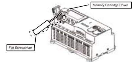
After removing the memory cartridge cover, check that the triangular marks on the memory cartridge and the SmartAXIS point at each other to ensure that the memory cartridge is installed in the correct orientation.
