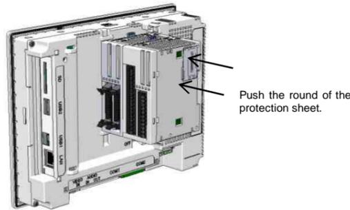
Procedure 3. Fix the expansion modules by pushing down the disassembly buttons to the same position as the expansion module's upper side.
