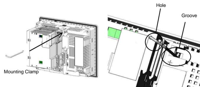
Procedure 6. Fasten the mounting clamp with the screw to a specified torque of 0.6 N·m pushing the mounting clamp as shown in the following figure. After fastening the mounting clamp, make sure that the mounting clamp is not loose and not having a gap.
