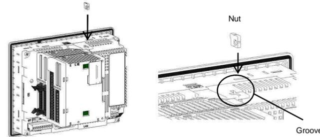
Procedure 5. Insert the A side of the mounting clamp into the groove. And hook the B side of the mounting clamp on the hole of the expansion module.
