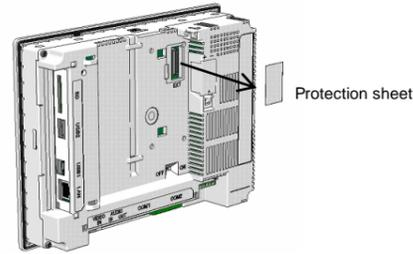
Procedure 2. Unlock disassembly buttons of expansion modules and then push the expansion modules into the back of the HG making sure of the position of the expansion module's connector. Push the round of the protection sheet of the expansion modules. And make sure there are no gaps between the HG and the expansion modules. Also make sure there are no gaps between expansion modules when using two or more modules.
