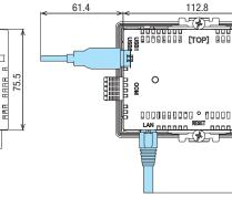
• Dimensions in blue show the mounting dimensions of the cable. USB and LAN interfaces are as shown in the dimensional drawings above. When installing, take into consideration the space required for your USB device or LAN cable.
