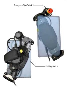
\*) The above image shows the device mounted on a commercially available tablet.
