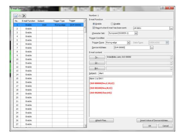
To insert PLC/HMI data register addresses in the email body to display dynamic data, click "Insert Value of Device Address" on the Email Settings
