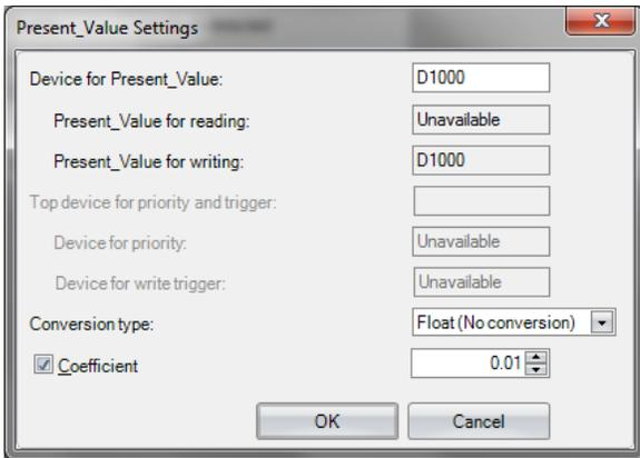
This means that the value we are providing over BACnet is the value in D1000 multiplied by 0.01. In our case, we should see a value in YABE for the Analog Input object of  $1000 \times 0.01 = 10$ .
