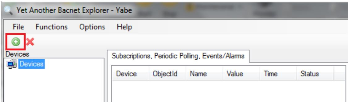
This will bring up the Search dialog box. In the BACnet/IP over Udp section, set Port to BAC0 and Local endpoint to the IP address of the Ethernet port on your computer that you are using to connect to Ethernet Port 2 on the FC6A Plus.
