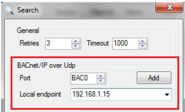
Click the Add button to search for BACnet/IP servers that are connected to the same network as 192.168.1.15.
