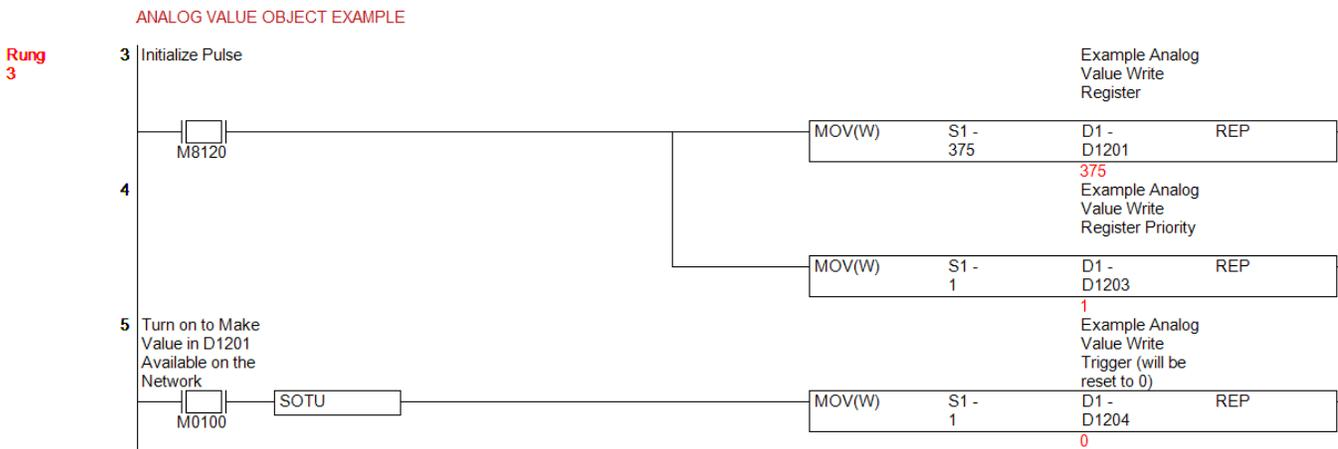
When we turn on M100, the value in D1201 will be made available to the BACnet/IP client. The value that the client is reading gets reported in D1200.
