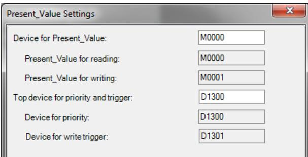
Device for Present\_Value is the starting internal relay for the Present\_Value for reading and Present\_Value for writing internal relays.
