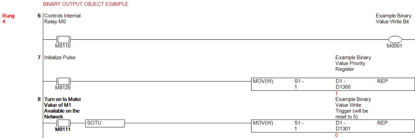
Internal relay M110 controls the status of M1. When we turn M111 on and off, it will make the status of M1 available to the network.
