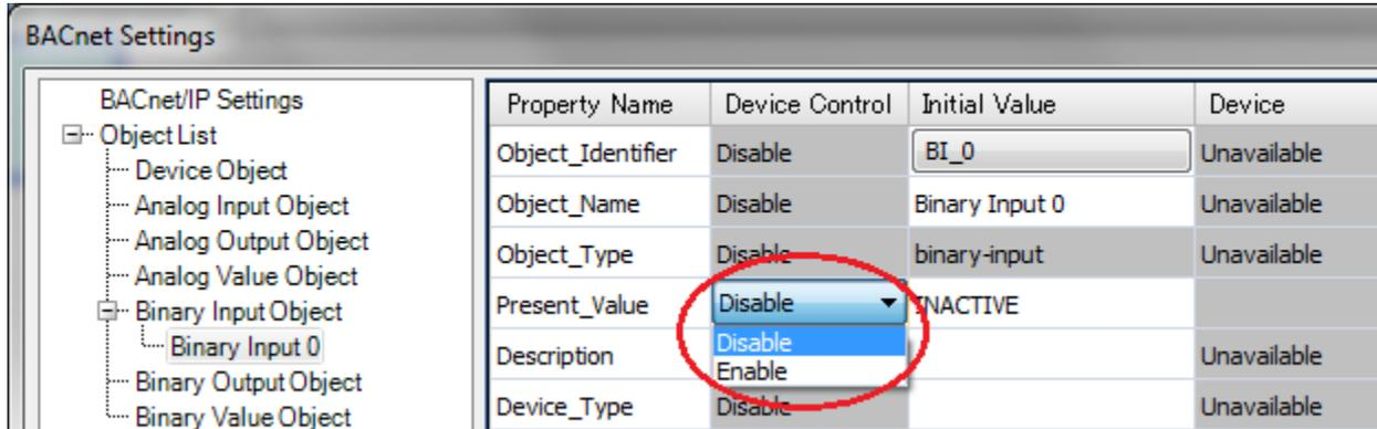
This will open up a button in the Device column. Click the **button** under Device column.
