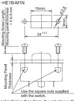
Note: When installed on a mounting panel is thicker than 2mm, the actuator surface is below the panel when the actuator is pressed to the bottom.(HE1B-M1N)
