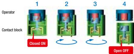
When the contact block is detached from the operator, the cam directly opens the NC main contacts (contacts are off). (Patented)
